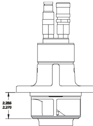
*Figure 7-1. There should be an offset of between 2.270 and 2.285 inch from the bottom of the motor flange to the bottom of the stepped diameter.*
