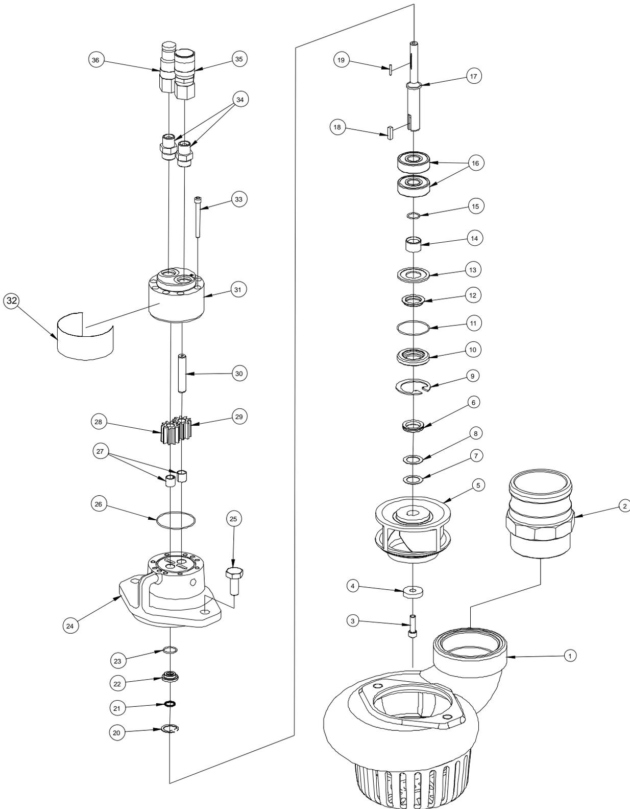
2. Remove the o-ring (26) from the motor cap.
