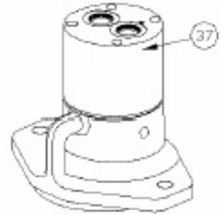
STN-65132 Motor assembly used on sump pumps with serial numbers 600 and above. This motor can only be purchased as an assembly; individual parts are not available.
