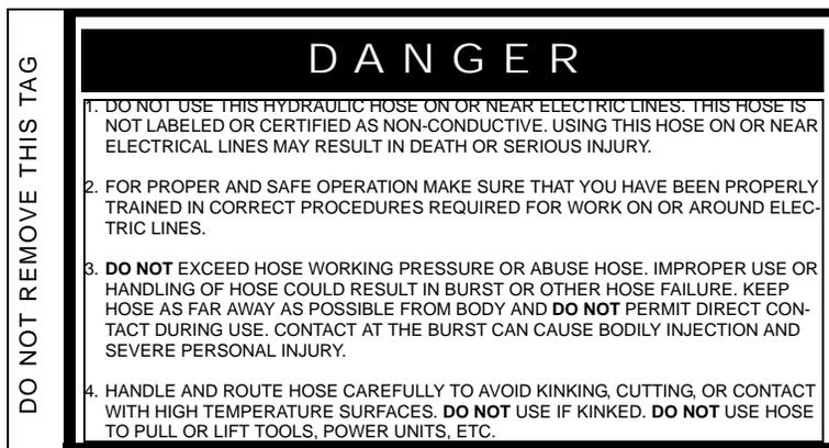
Figure 3-4. Tag attached to “Conductive” hose (front and back).
