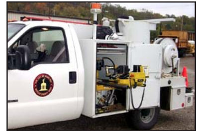
TM-7 valve operator with vertical tank Trav-L-Vac 300.
