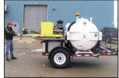
Curbside dump vac with 180° swiveling TM-7 valve operator.
