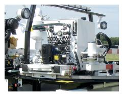
The TM-7 Swivel optional allows up to 15 degrees of valve stem misalignment
