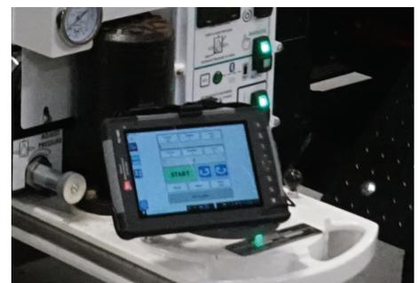
The ruggedized TC-100 handheld computer / wireless controller / datalogger provides intuitive remote exerciser control
