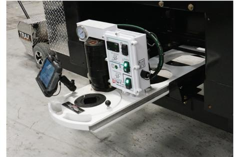
TM-7 HD Plus valve operator provides 2500 ft-lb of torque for turning large valves
