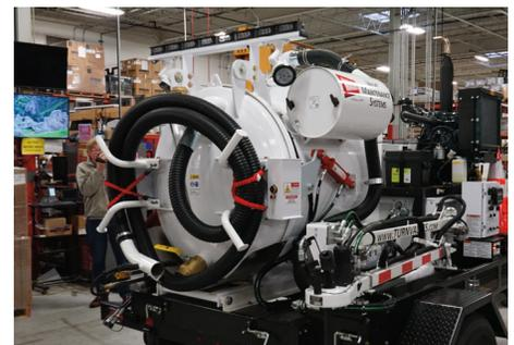
The heavy-duty spoils tank features a two-cylinder electric over hydraulic slide, tilt and dump functionality for easy emptying
