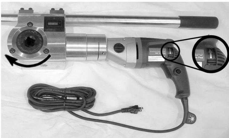
Figure 1-3. The photo illustrates the direction of rotation for indicated motor direction.
