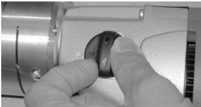
*Figure 3-6. Turn the gear ratio switch to the speed range desired.*
