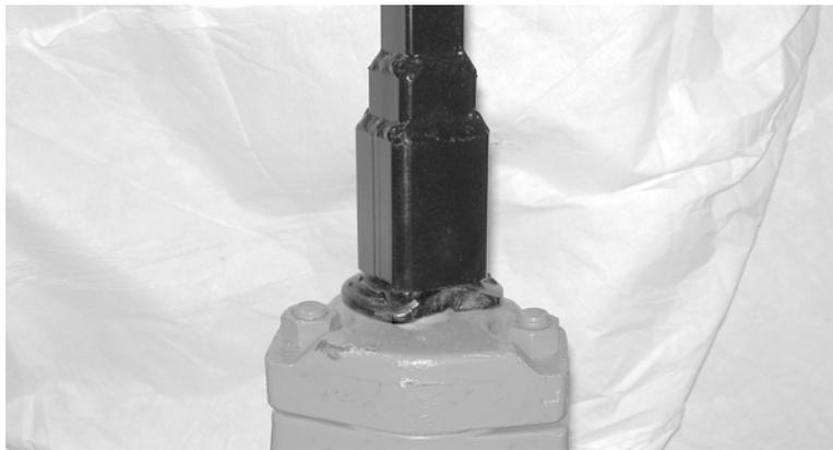
*Figure 3-2. Put the socket onto the valve nut.*
