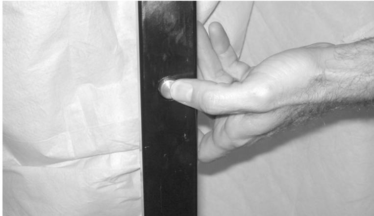
*Figure 3-1. Press in the locking pin to adjust the length of the valve key.*
