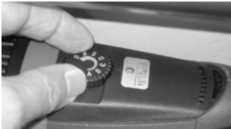
*Figure 3-5. Turn the speed dial to increase the speed.*
