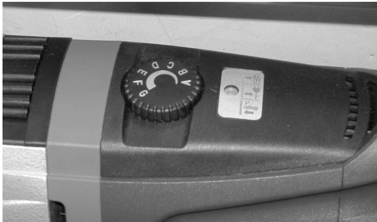
*Figure 3-4. Start with the speed dial set to the lowest speed (“A”).*
