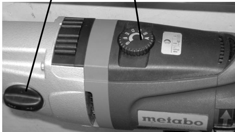
*Use the speed control dial and the gear ratio switch to set the electric drive speed.*
