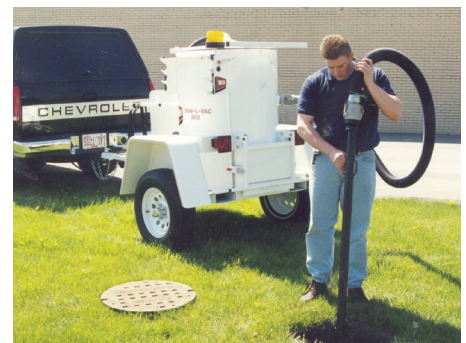
Steel suction tube with handles allows the operator to effortlessly guide debris removal
