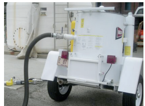
Large capacity holding tank with manually activated dump gate makes emptying simple
