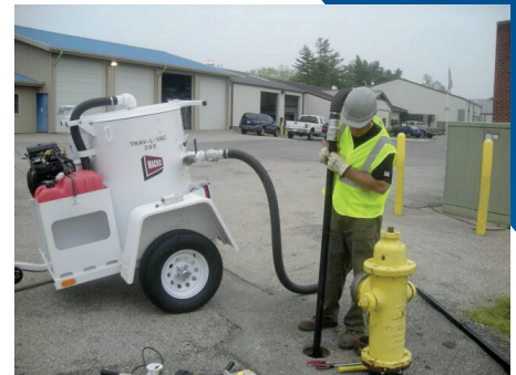
10ft flexible wire-reinforced rubber suction base hose makes reaching the valve box easy
