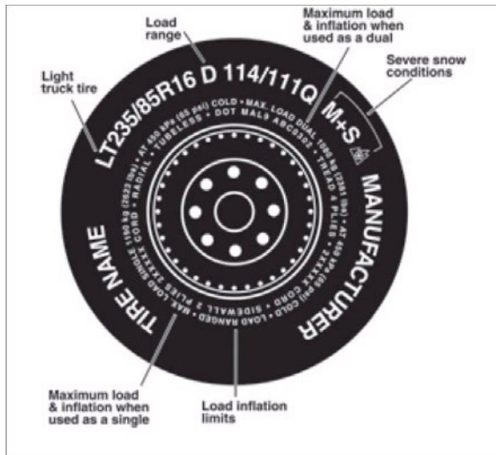
**Max. Load Dual kg (lbs) at kPa (psi) Cold:** This information indicates the maximum load and tire pressure when the tire is used as a dual, that is, when four tires are put on each rear axle (a total of six or more tires on the vehicle).
