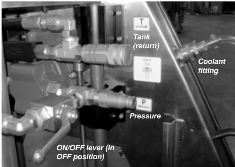
*Figure 1-5. The photo shows the fittings and controls on the machine.*
