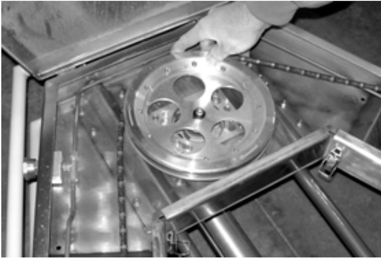
Figure 4-3. Remove the wire from the drive wheel first.
