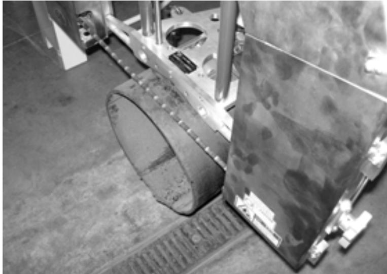
*Figure 3-12. Feed the bow down until the wire almost touches the pipe.*
