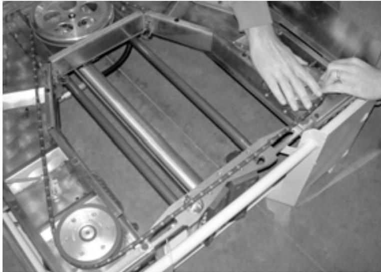
*Figure 4-5. Put the new wire over the wheels.*
