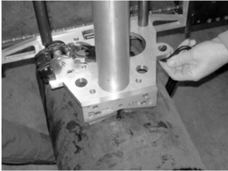
*Figure 1-4. A clamping strap with a ratcheting clamp holds the machine to the pipe.*
