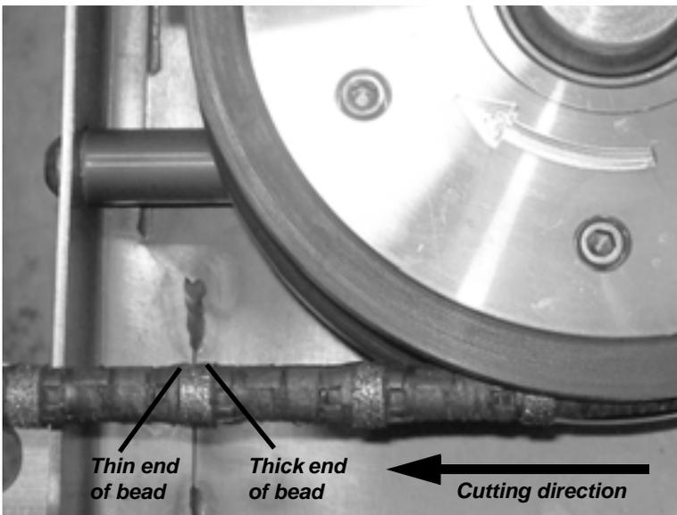
Figure 4-4. Check that the wire is installed in the correct direction. The thinner end of the cutting bead should lead.
