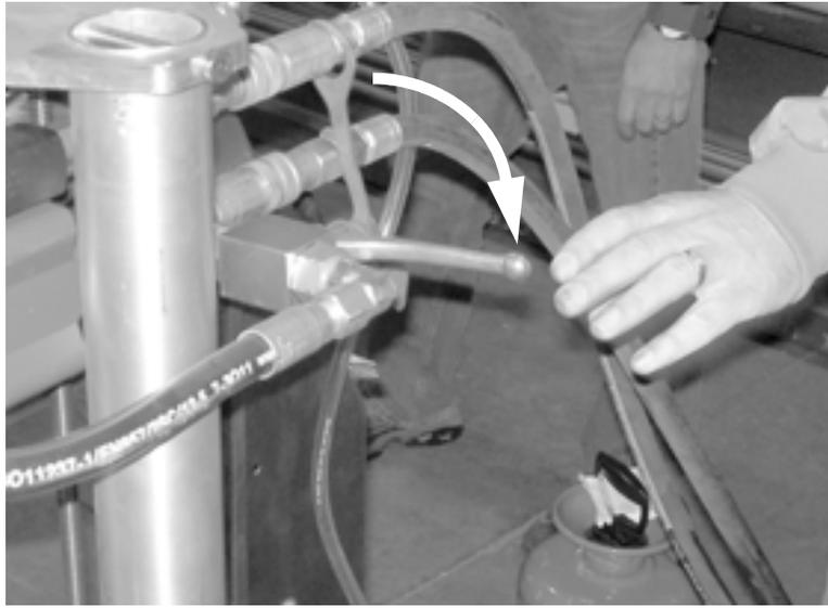
*Figure 3-19. Turn the ON/OFF lever to the OFF position.*
