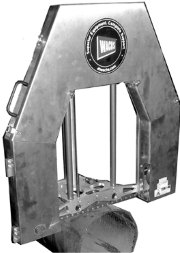
*Figure 1-1. The photo shows the DW Guillotine mounted and ready to cut.*
