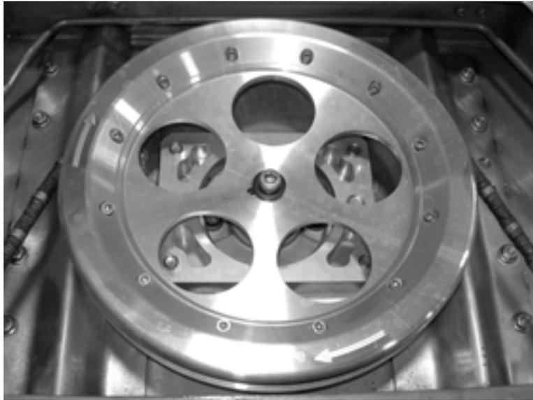
*Figure 4-8. The drive wheel has 12 screws holding the cover*
