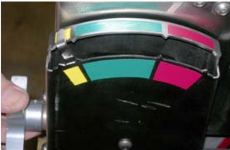
*Figure 3-11. With no load on the wire, the tension gauge indicator should be in the yellow.*
