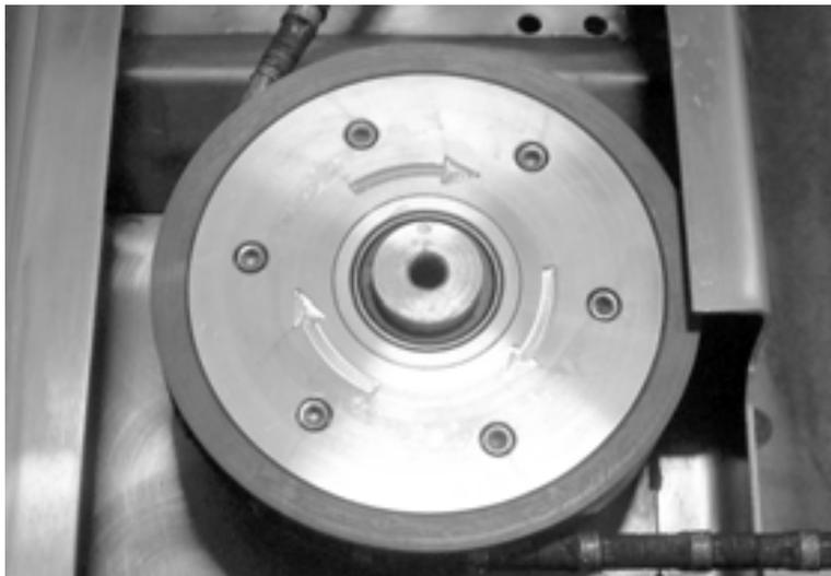
*Figure 4-7. The idler wheels have 6 screws holding the cover.*
