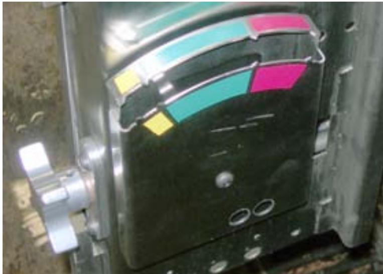
*Figure 3-17. Operate the feed handle to keep the tension gauge indicator in the green band.*
