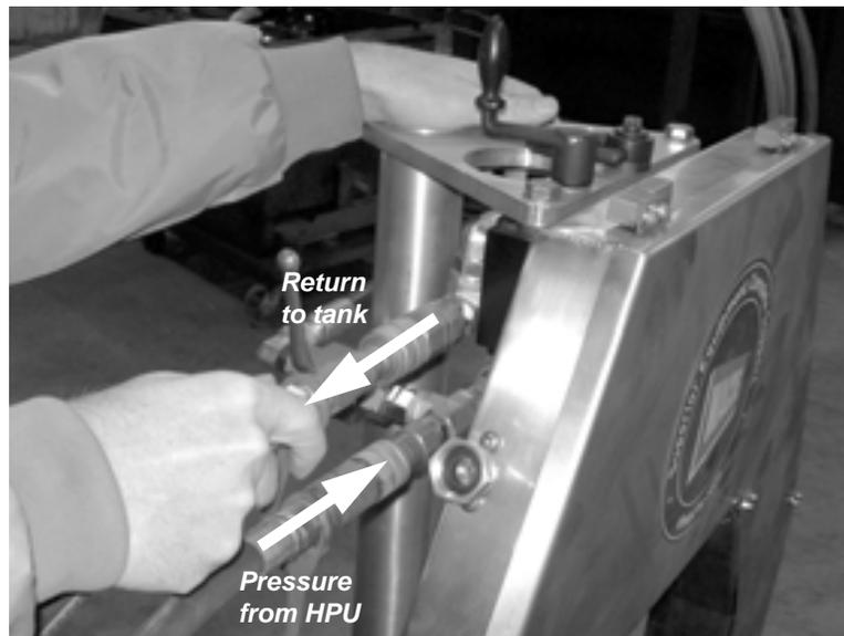
Figure 3-9. Connect the hydraulic hoses.
