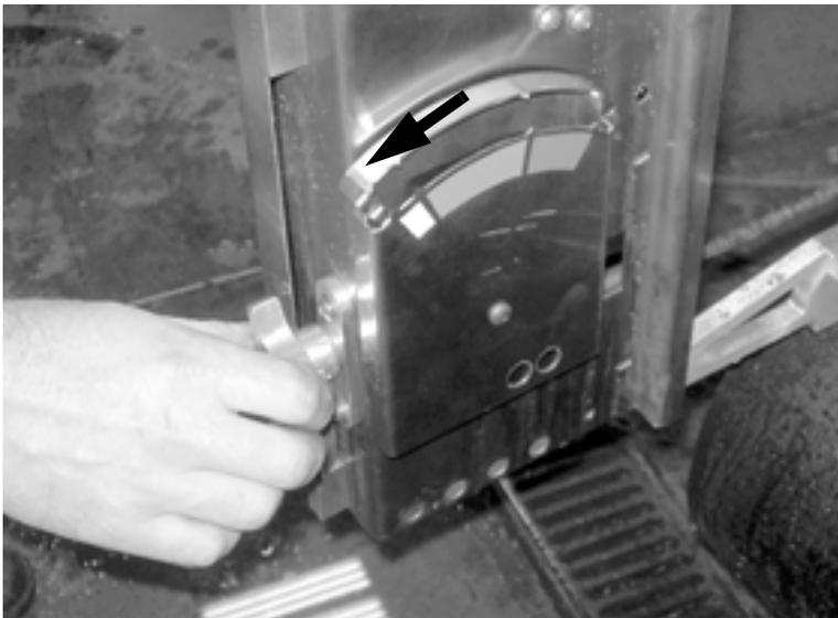
*Figure 3-21. Loosen the tension knob to take the tension off the wire. The tension gauge indicator should be all the way to the left (below the yellow band).*
