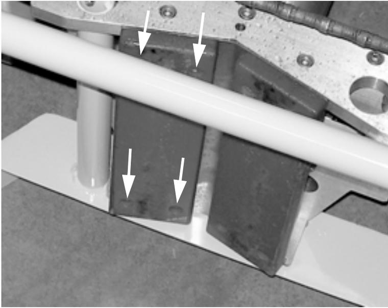
*Figure 4-9. Each mounting shoe is held on with 4 screws. Remove the screws to replace the shoe.*
