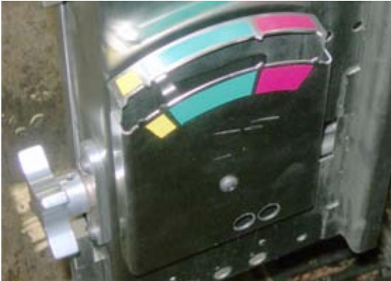
*Figure 1-6. The tensioning gauge monitors the tension on the wire as it cuts.*
