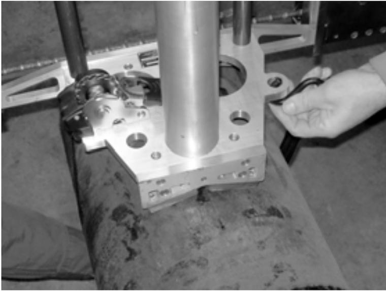
*Figure 3-6. Wrap the clamping strap around the pipe and fasten the hook through the hole as shown.*
