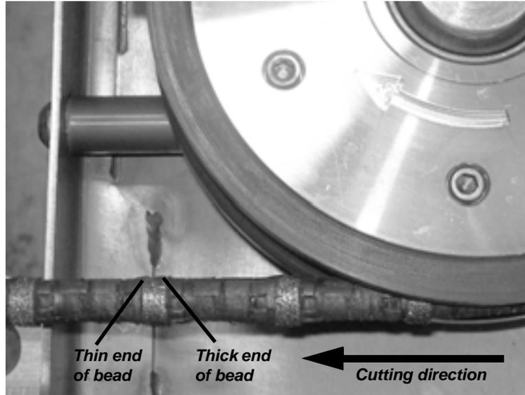
Figure 3-8. Check that the wire is installed in the correct direction. The thinner end of the cutting bead should lead.
