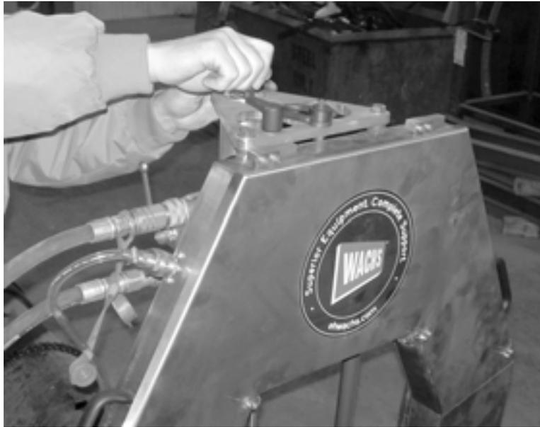
*Figure 3-16. Turn the feed handle to advance the wire into the pipe.*
