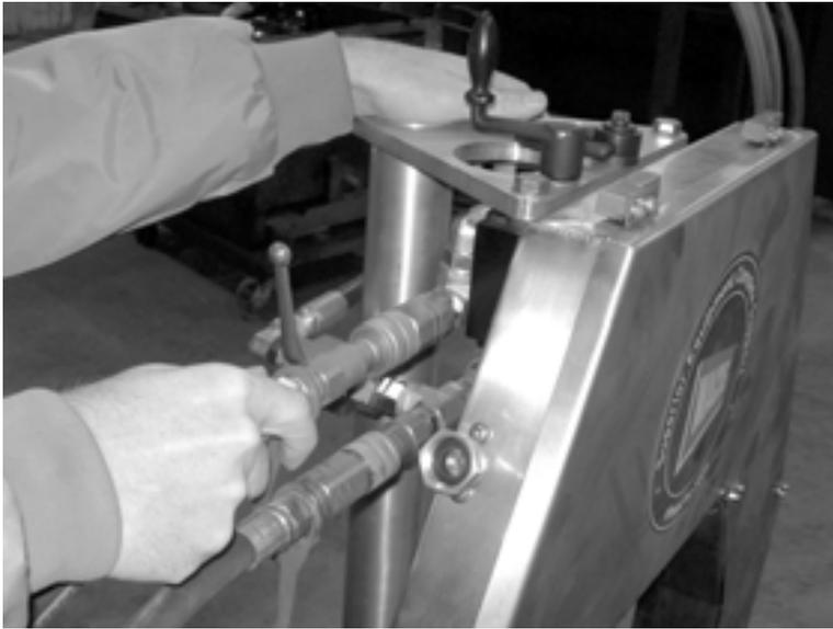
*Figure 3-20. Remove the hydraulic hoses from their fittings.*
