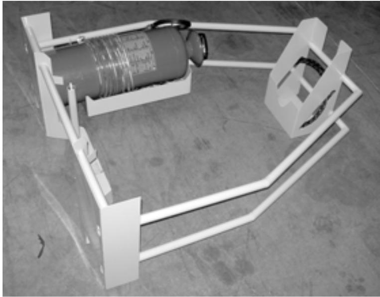
*Figure 1-7. A storage stand is provided to hold the machine and accessories. The coolant sprayer provides water for cutting lubrication.*
