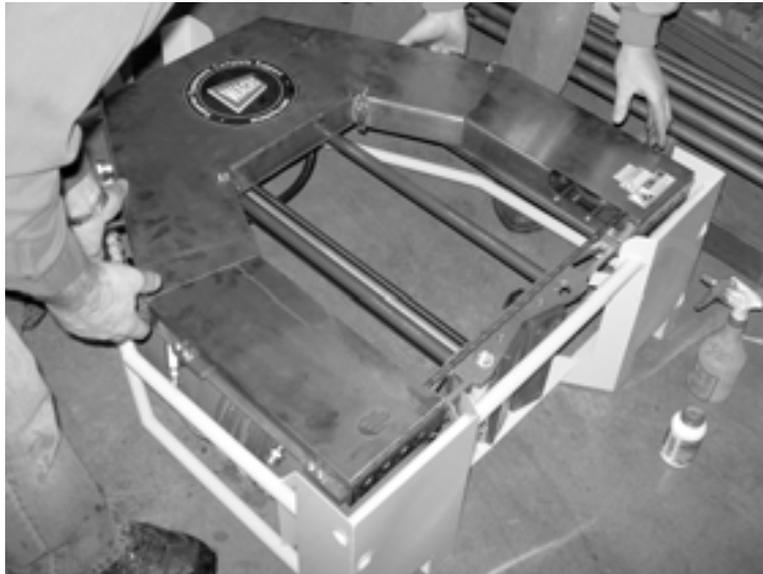
*Figure 3-2. Lift the machine out of the storage frame.*
