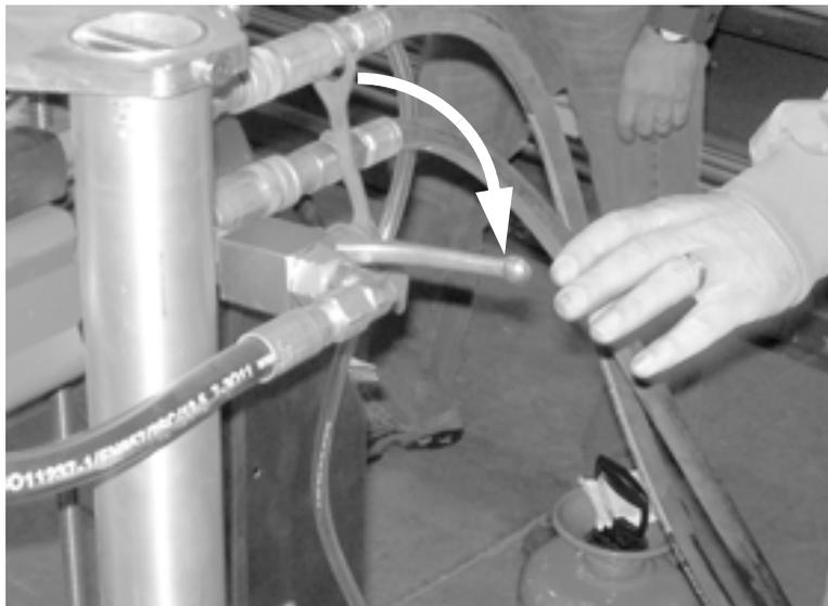
*Figure 3-13. Make sure the machine is turned off before starting the HPU.*
