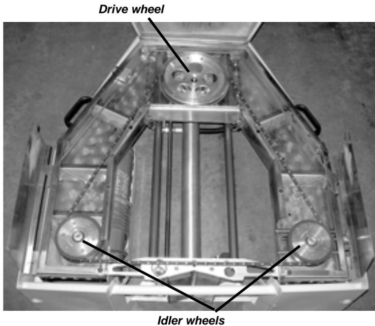
*Figure 4-6. Open the covers to access the wheels.*
