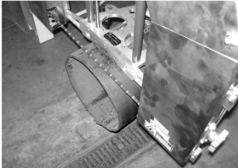
*Figure 3-4. Position the machine so the wire is at the cut line location.*
