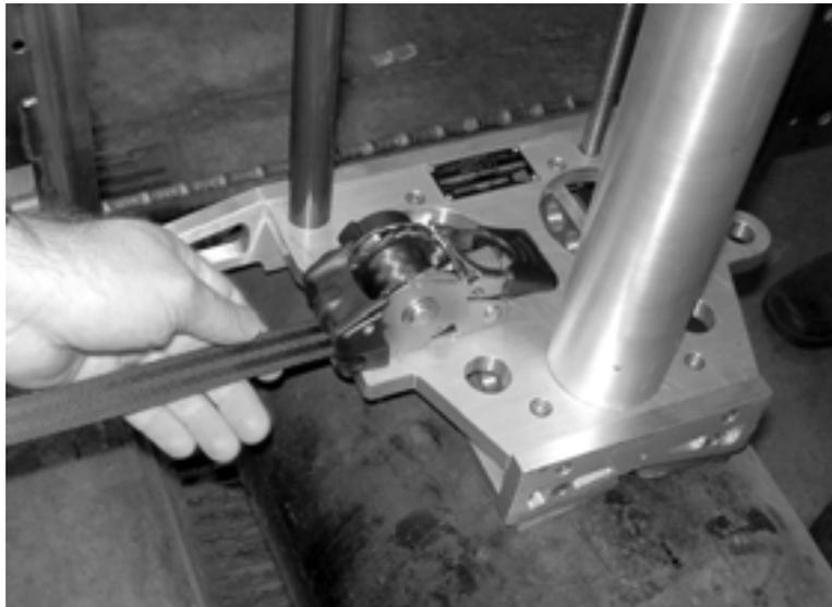
*Figure 3-5. Pull out enough strap to wrap around the pipe*
