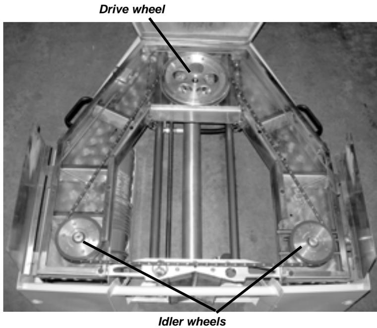
*Figure 1-2. The drive wheel runs on the shaft of the hydraulic motor. The idler wheels spin freely with the motion of the wire.*
