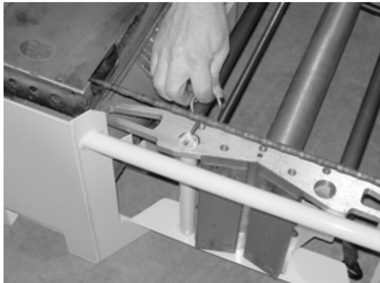
*Figure 3-26. Put in the locking pin to secure the machine in the storage frame.*
