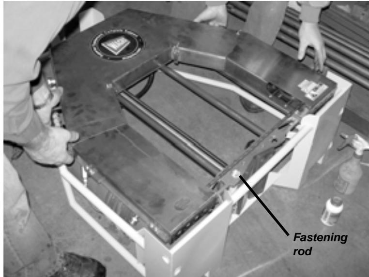
*Figure 3-25. Set the DW Guillotine down in the storage frame.*
