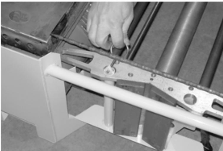
*Figure 3-1. Pull the locking pin out of the fastening rod.*
