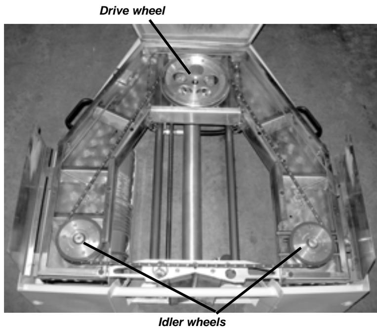
*Figure 4-2. Open the covers to access the wire.*
