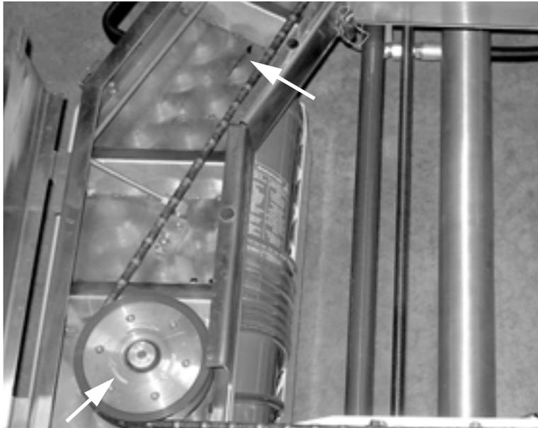
*Figure 1-3. Direction arrows on the wheels and frame show the direction of wire rotation.*
