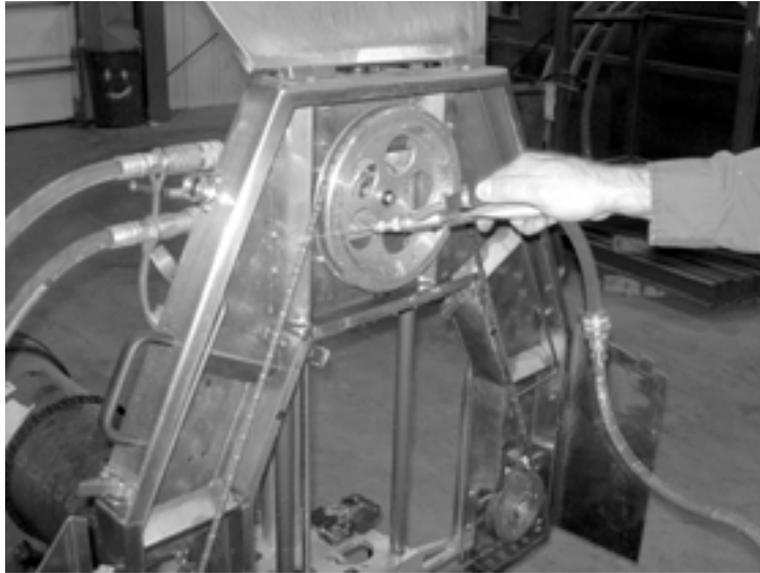
*Figure 3-22. Spray the inside of the machine thoroughly to clean out cutting debris.*
