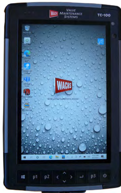
Figure 3-2. The TC-100 handheld controller is a fully functional Windows 10 computer, running Vitals Mobile software.
