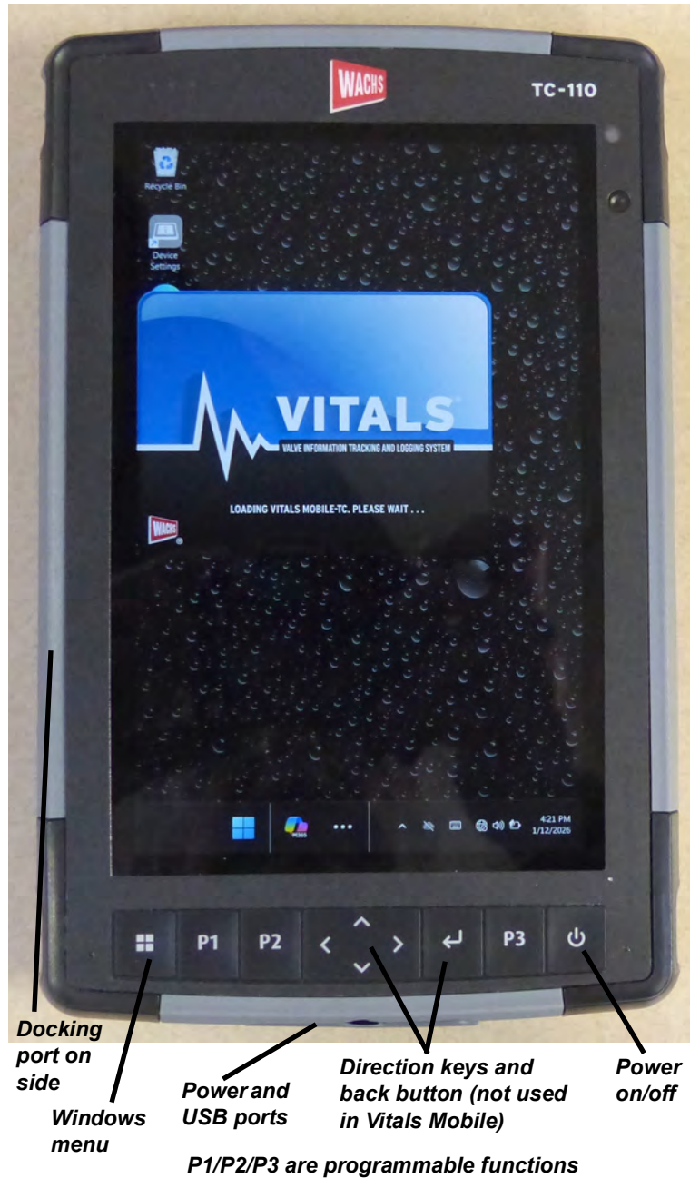
Figure 5-1. TC-110 connections and control buttons
