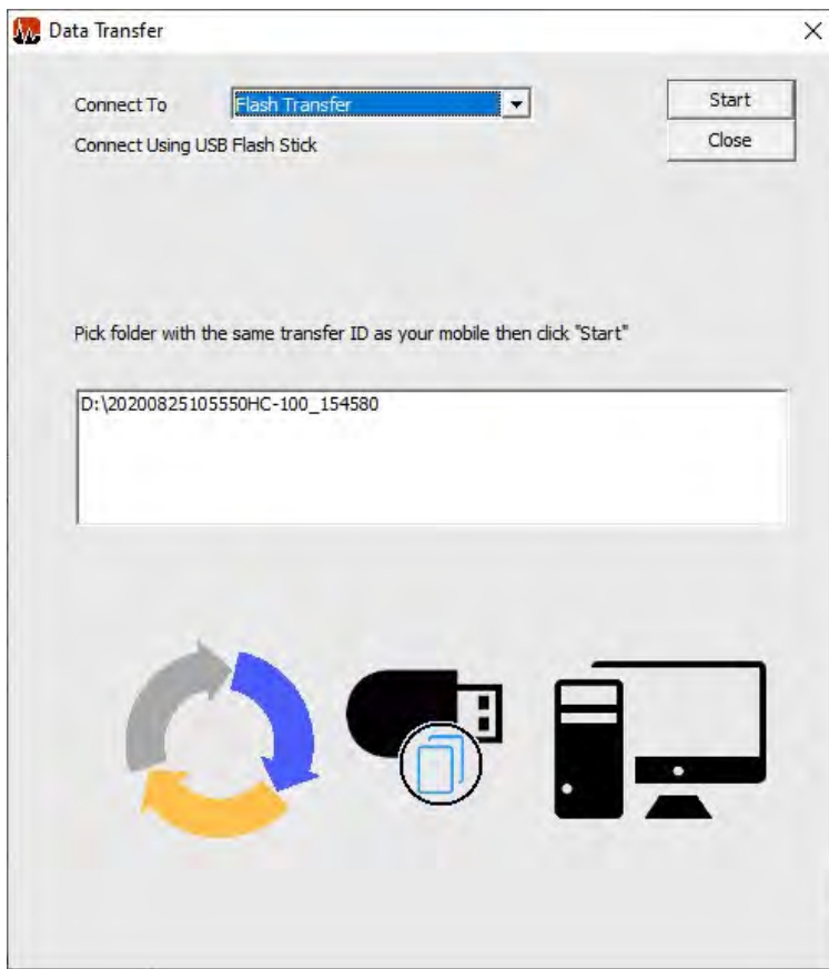
Figure 7-43. Select the name of the folder in the window. (Multiple folders will appear if there are transfers from multiple handheld controllers on the USB flash drive.)
