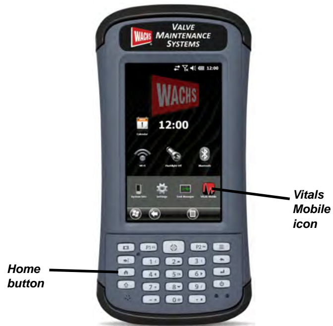
Figure 6-1. HC-100 home screen. Press the Home button on the keypad at any time to return to the home screen.
