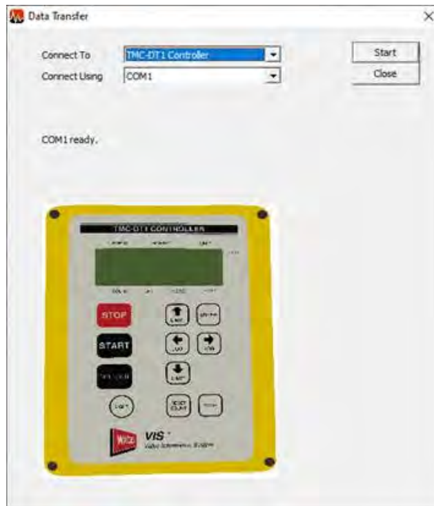
Figure 7-50. Data Transfer Start Screen for Yellow TMC-DT1 Controller.
