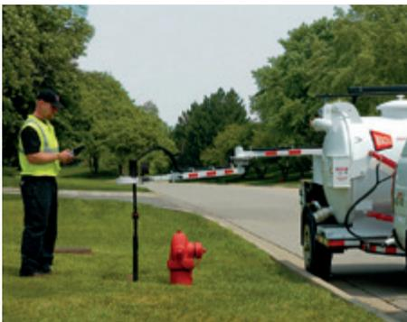
ERV-750 extended reach valve exerciser allows valve operation from the road
