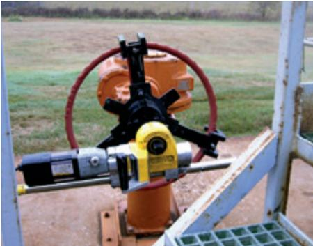
Pow-R-Drive 2 Handheld Valve Exerciser shown with optional handwheel adapter
