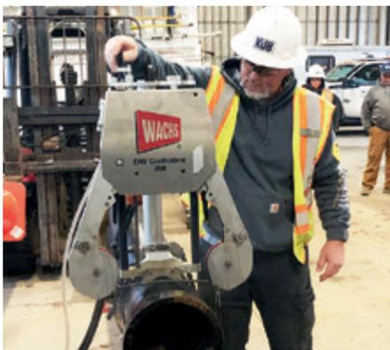
Mounts directly to workpiece for easy single operator use
