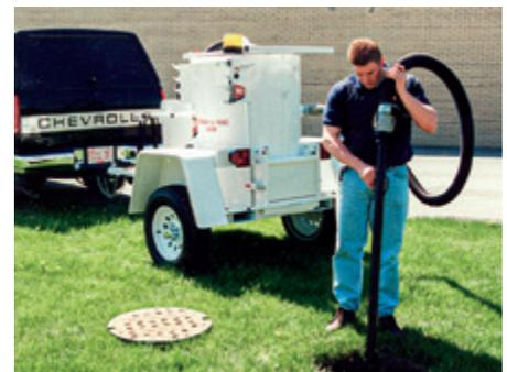
Steel suction tube allows the operator to effortlessly remove debris
