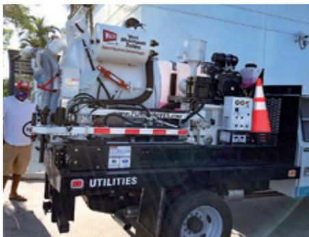
Skid system allows for simple mounting to a flatbed truck.
