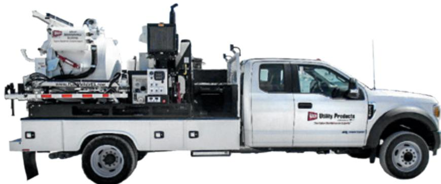
Knapheide / Wachs Valve Maintenance Truck Service Body with Integrated Wachs Service Body Valve Maintenance Skid
