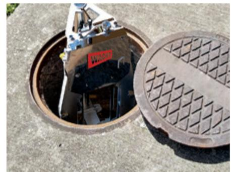
DWG 416 is designed to collapse and fit inside of utility access holes
