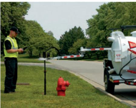
ERV-750 easily reaches any curbside valve box or hydrant within 13 feet of the mount
