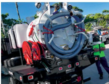
250 gallon spoils tank utilizing exclusive hydraulic slide, tilt & powered dump system
