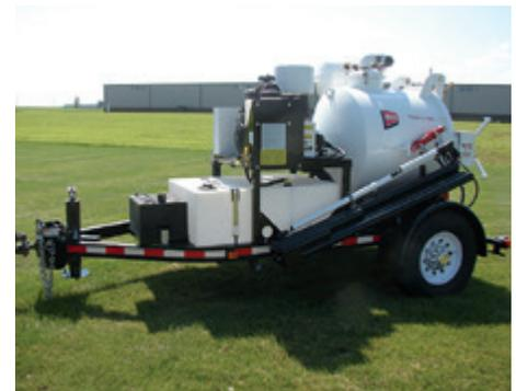
Power pack provides pressure washer system and 500CFM vacuum
