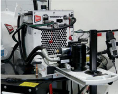
TM-7 SD Plus valve operator provides 1500 ft-lb of torque for rehabilitating larger valves
