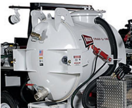
The heavy-duty spoils tank features power tilt and dump for easy emptying
