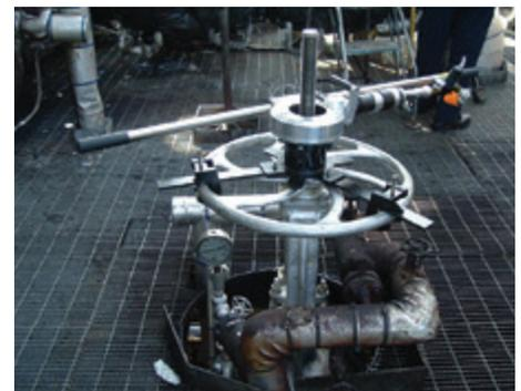
RS-2 shown with optional universal handwheel adapter on a rising stem valve
