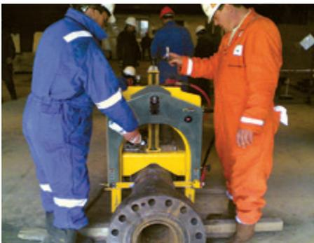
Guillotine saws feature fast, easy operation and the ability to cut most materials
